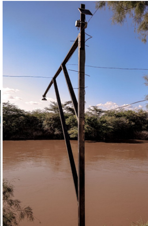
Figure 4.24: MoEWR dashboard showing the Radar Water Level Sensor: RLS001 - Beledweyne at Shabelle River.
